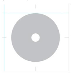
Outer diameter 117 to inner diameter 20 mm
